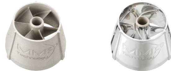
Fuel air swirler before and after MMP surface treatment
