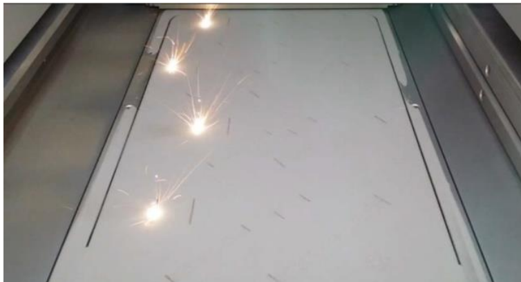
Image of the manufacturing chamber of SLM Solution's SLM 500 PL system capable of using 4 independent lasers and scanner systems simultaneously
