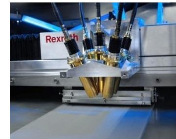
View of the processing head: a five-spot array is mounted on a single scanning head
