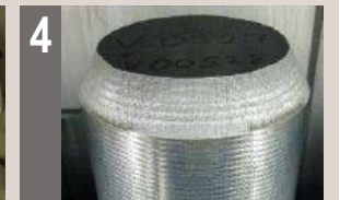
4) Dissolving of carrier material in cooling channel
