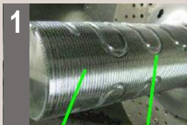
1) Milling of cooling channel in raw material
