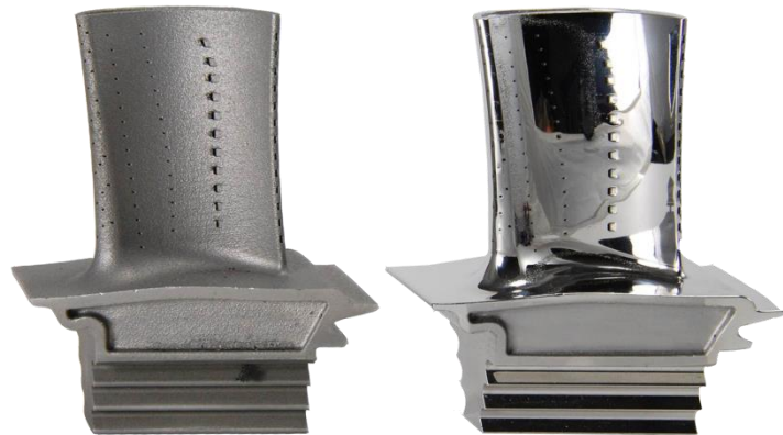
AM turbine blade, before and after surface treatment
